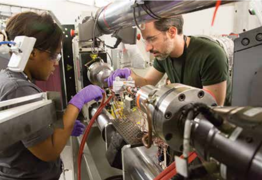
Top: Protons accelerated by this underground linear accelerator at Oak Ridge National Laboratory are collided with a mercury target, generating high-energy pulses of neutrons that are directed into multiple beamlines for research into the properties of materials. (Genevieve Martin / Oak Ridge National Laboratory)
