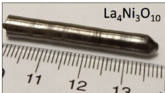
Figure 3.6.2: High pressure image furnaces have recently been developed, opening up a large parameter space that was previously inaccessible for the synthesis of new materials. The photograph shows a large single crystal of the trilayer nickelate \text{La}_4\text{Ni}_3\text{O}_{10} grown in 25 bar \text{O}_2 using such a furnace. Much higher gas pressures are in principle possible if combined with a laser diode furnace, since the windows can be much smaller. Photo courtesy J. Mitchell.
