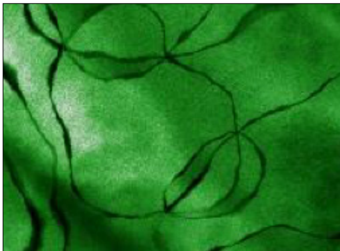
Figure 2.4.3: Topologically protected quantities are not just associated with electronic states. Domain wall configurations in certain low-symmetry structures are also topologically protected and their density can be controlled during the growth process. The figure (courtesy S.W. Cheong) shows a transmission electron microscope image of structural domain walls in multiferroic \text{ErMnO}_3 . The topology of this structure ensures that six domain walls meet at each vortex.
