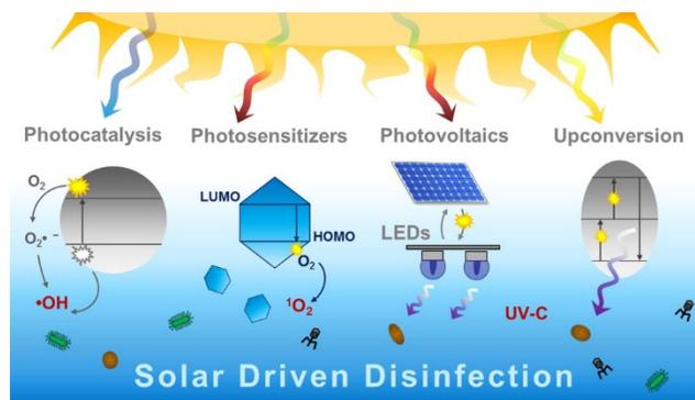
Figure 3.3.6. Advanced technologies for solar energy disinfection.
