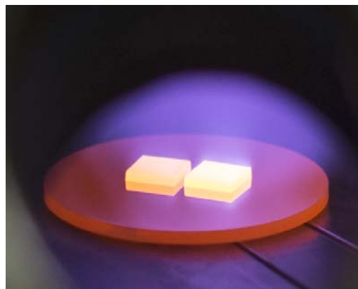
Figure 4. Diamond homoepitaxial growth. Courtesy of Bob Nemanich and Franz Koeck, Arizona State University.
