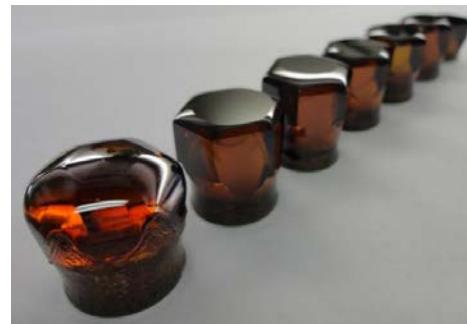
Figure 3. Array of 25-mm AlN boules used to make substrates for epitaxial growth. Although substrates up to 2-in. dia are commercially available, larger substrates are needed for economic feasibility. Courtesy of Greg Mills, HexaTech.
