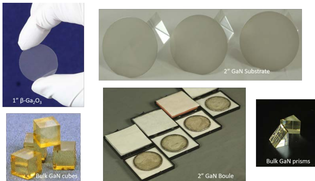
Figure 2. WBG and UWBG substrates. Courtesy of Jacob Leach, Kyma Technologies.
