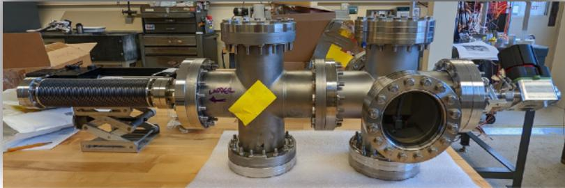
Offline assembly & testing of diagnostic target drive
