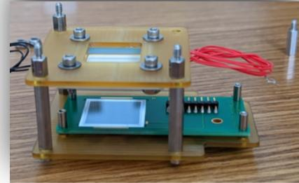
Particle identification + positioning detector system
