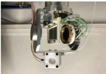
Passive detection of beam positioning [ $\sim 1$  mm] & timing [ $< 1$  ns] event - by - event
