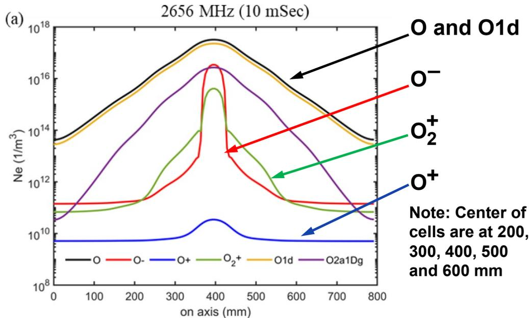
Simulation based spatial distribution of different species of oxygen (molecules, ions, and metastable states) on the axis for one of the modes in a C75 cavity.\*
