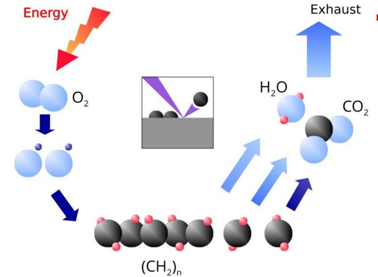
O<sub>2</sub> is cracked in the plasma to atomic oxygen which breaks down the hydrocarbons
