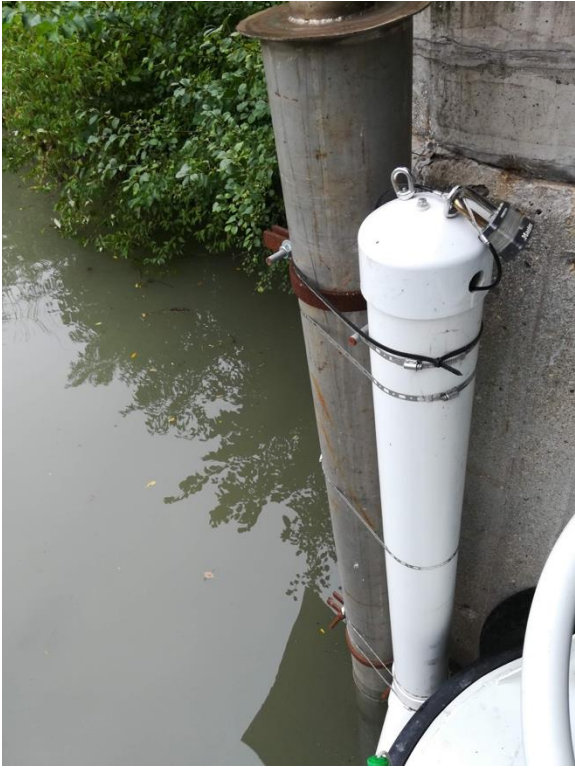
Figure 1. Example housing for water quality sonde.
