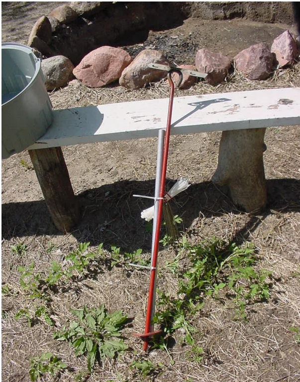
Example affixment for flowmeter sensor and autosampler tube.
