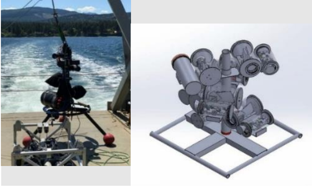
Figure 2.2. Versions of the UMSLI Developed by Florida Atlantic University, Approximately 81 cm (32 in.) Tall, 107 cm (42 in.) Wide.
