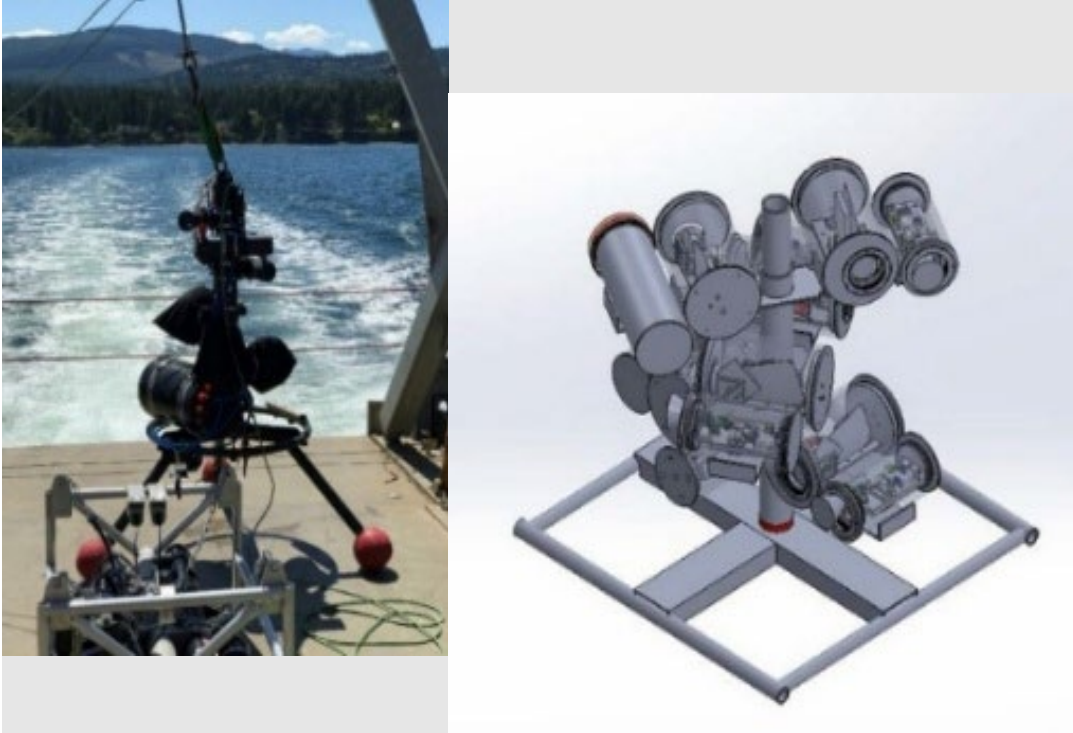
Figure 4. Versions of the UMSLI developed by Florida Atlantic University; approximately 81 cm (32 in.) tall, 107 cm (42 in.) wide.
