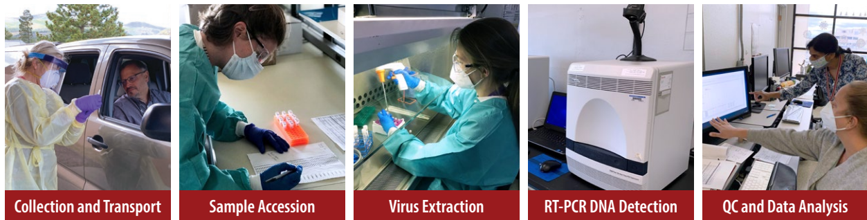
Fig. 8. The nucleic acid testing process involves five phases, outlined above. [Courtesy Los Alamos National Laboratory]
