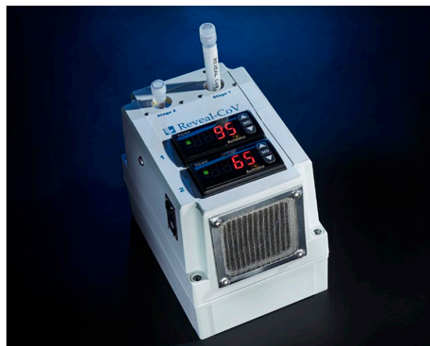
Fig. 10. Reveal-CoV uses Reverse Transcription Loop-mediated isothermal AMPLification (RT-LAMP) to rapidly detect SARS-CoV-2. An initial inactivation step is performed at 95°C followed by amplification of the target sequence at 65°C and visual detection of color change. Total time from sample to answer is less than 1 hour. [Courtesy Lawrence Livermore National Laboratory]
